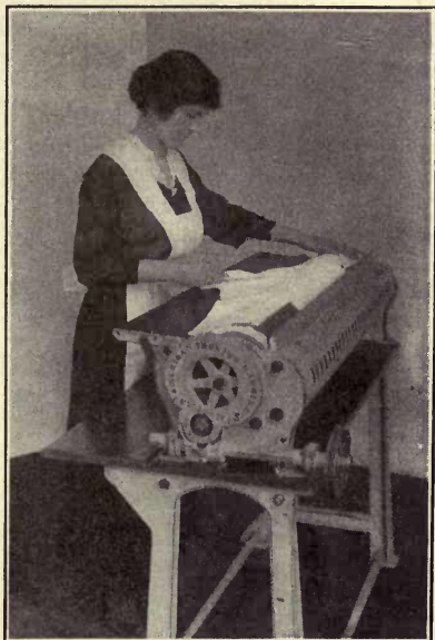
FIGURE 185.—ELECTRIC IRONING MACHINE. HEATED AND RUN BY ELECTRICITY.
